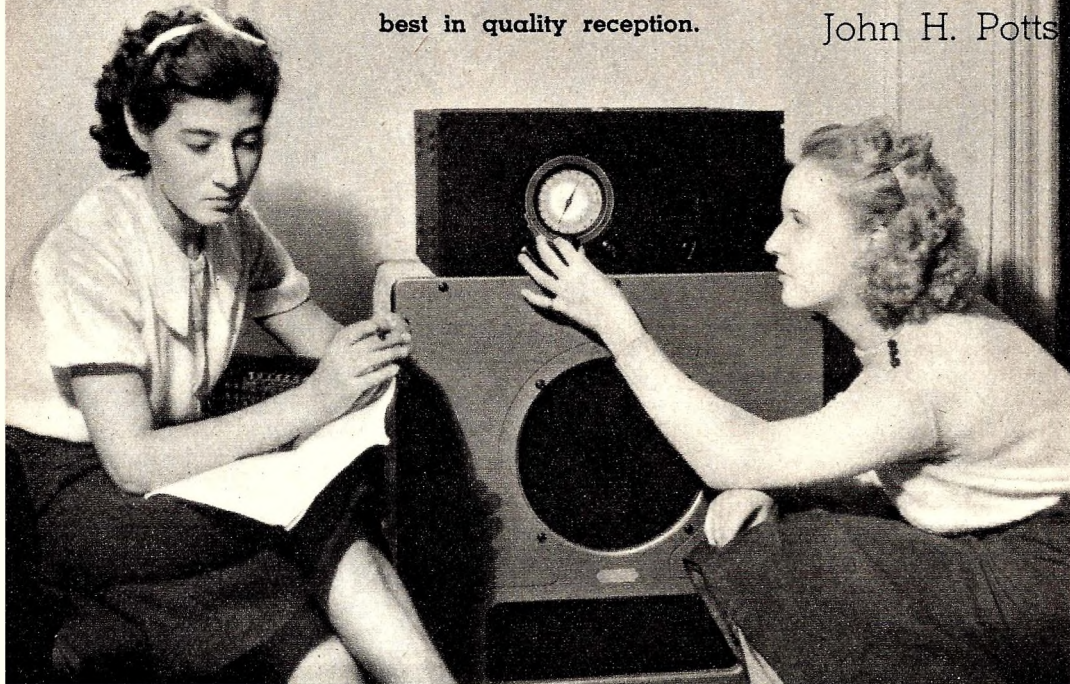
This photograph shows the completed receiver in operation. The receiver itself is contained in the metal cabinet on the speaker. Although a steel panel can be used, one of aluminum will be much easier to drill.
