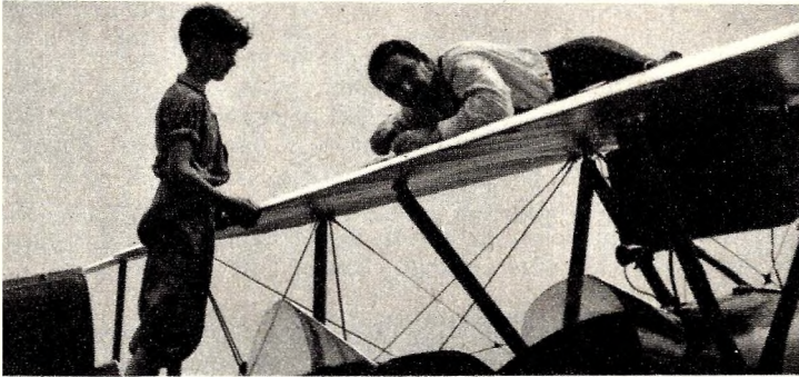
Inspecting a plane before renewing its license, the inspector climbs atop the wing to examine it minutely for flaws. Planes are inspected at regular intervals.
