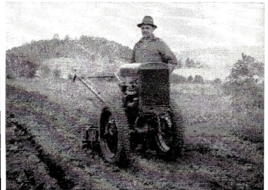
Parts salvaged from old autos and trucks were converted into this practical hand-guided garden tractor by A. H. Barsie.
