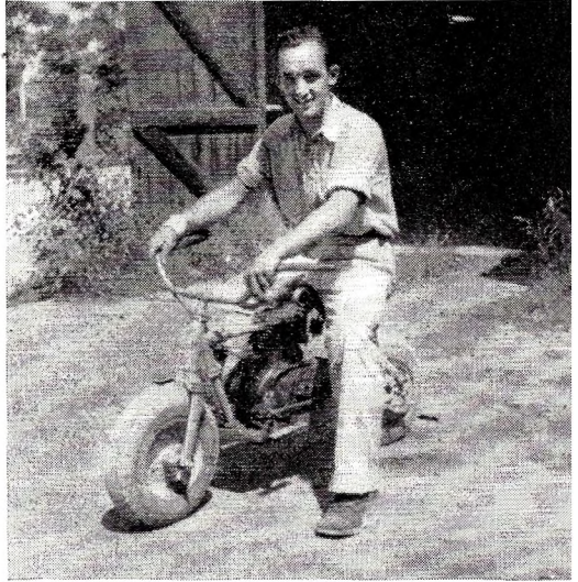
There is plenty of appeal in the midget motorcycle constructed by A. M. Harley. Powered by a one-half horsepower motor, it has a frame made from iron pipe welded together at the joints.
